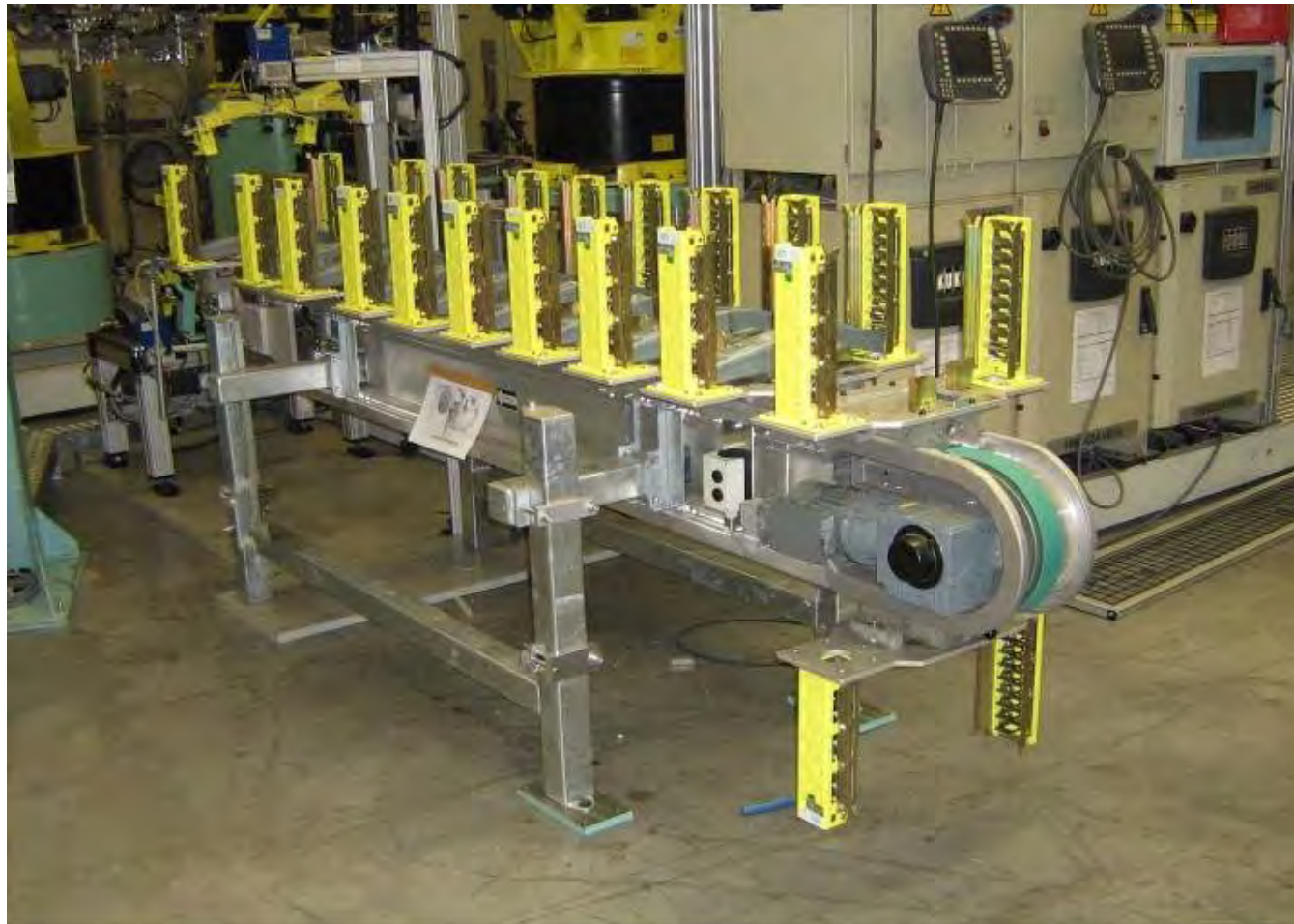
LFS-LAT Conveyor System
