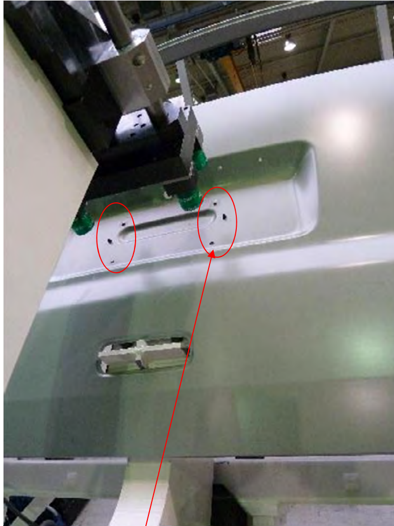
Piercing of 4 holes SW 9,0 mm in 0,8 mm thick steel sheet
